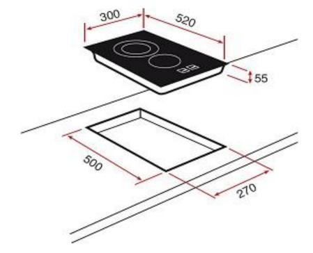
ATTENTION: Cut hole must be with round corners in order to avoid cracking on the counter-top.
